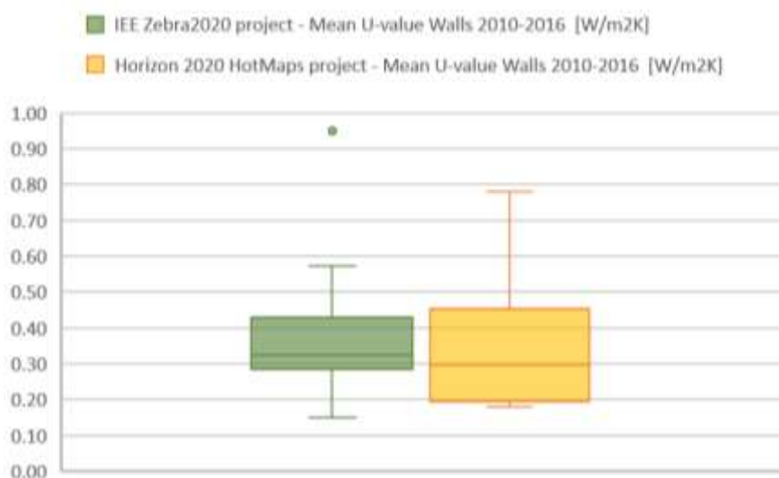
Figure 2: Quality control level 3 main statistical data - graphical representation - datasets comparison number 4 [15], [11] according to Table 2. For more information concerning the datasets used please see Deliverable D3.1 of BuiltHub [2].
